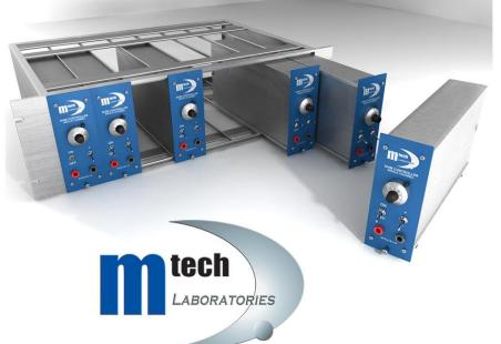
The current controllers can be configured for any number of channels. Each channel features a manual current adjustment, on-off switch, and polarity switch. Current can be adjusted by a 10-turn front panel potentiometer or by an analog signal (0-10 volts) for remote computer control. The controllers require a DC power supply, which can be provided as an option.
