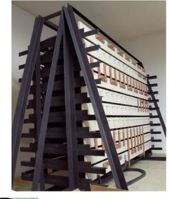
A power resistor block installed for testing high-power converters for the Navy.
