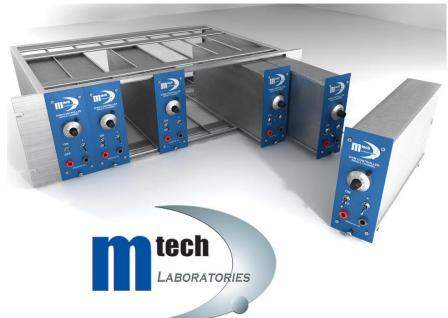
The shim controllers can be configured for any number of channels. Each channel features a manual current adjustment, on-off switch, and polarity switch. Current can be adjusted by a 10-turn front panel potentiometer or by an analog signal (0-10 volts) for remote computer control. The controllers require a DC power supply, which can be provided as an option.
